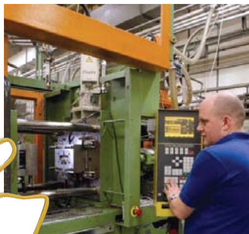
Top: Prav Mistry, machine setter, inspects a Kopex-Ex thread converter that's manufactured on a computer numerical control (CNC) machine at the Coleshill Birmingham facility. A CNC machine is used for making metal parts for everything from car parts to construction parts.
